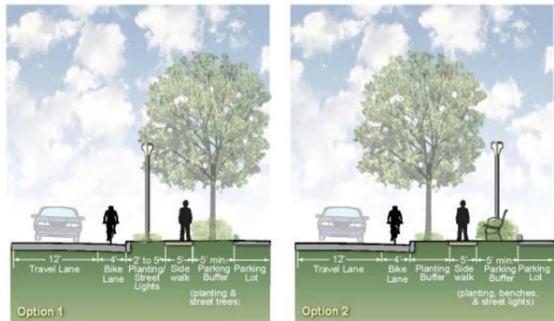
These examples show bike lanes and pedestrian buffers as a means to separate the different modes of travel.
