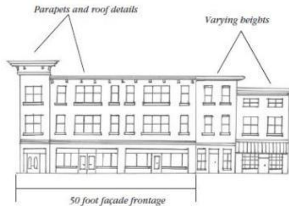
Variable roof heights and distinct details can help maintain building character along the whole façade. Source: Montgomery County Planning Commission
